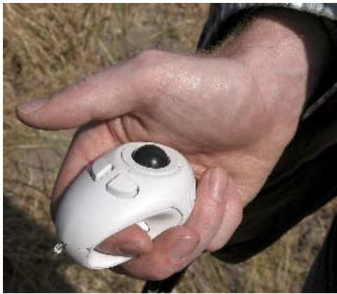
Figure 1: Finger Held Trackball Mouse
