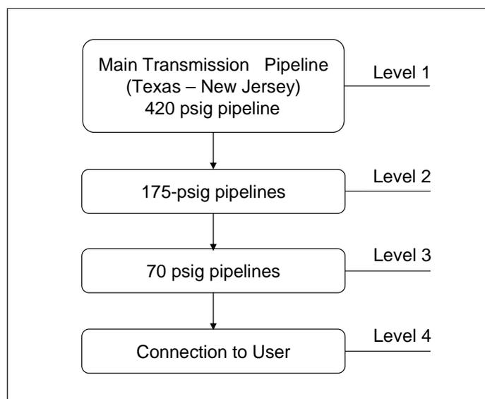
Figure 2. A functional hierarchy of the natural gas distribution system
