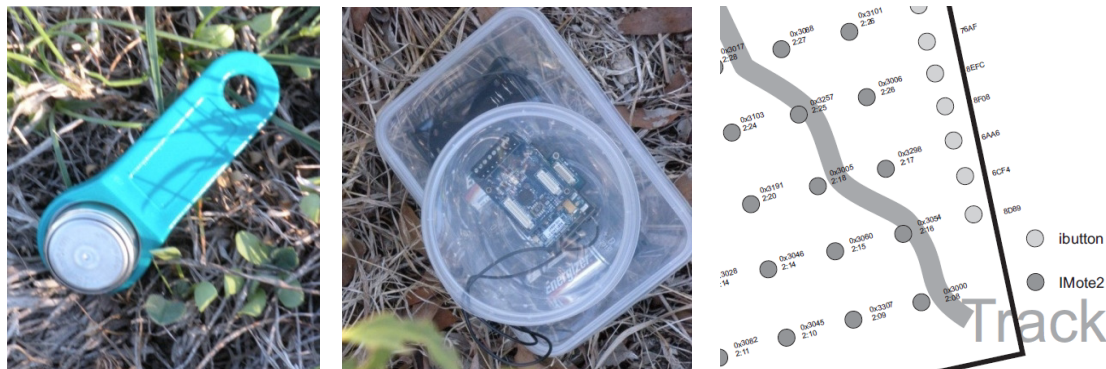
Figure 3: Sensor network nodes iButton (left) and iMotes (middle); part of the deployment map of site 2 showing approximate node locations (right)
